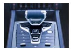
Push-type Electronic Gear Lever
